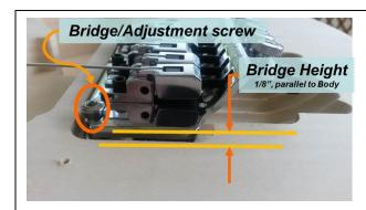
Figure 4.7-1 Tremolo String Installation
