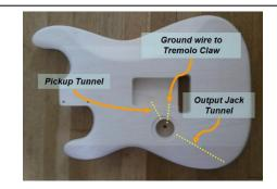
Figure 4.6.3-1 Body Wiring Tunnels
