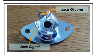
Figure 4.6.3-2 Output Jack Wiring
