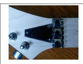
Figure 2.5.3 Truss Rod Cover
