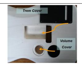
Figure 2.5.1 Back Body Cover Alignment
