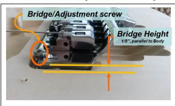
Fig 5.4 Action Adjustment
