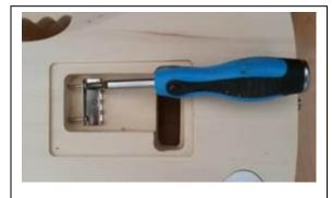
Figure 4.4-1 Tremolo Claw Installation
