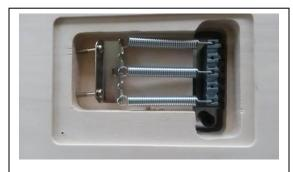
Figure 4.4-3 Tremolo Claw Installation
