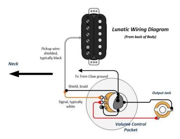
Figure 4.6.2-1 Lunatic Wiring Diagram
