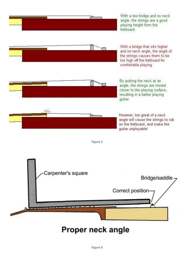
Now that you know where the neck should be located, all that's left is to glue it in place. Use yellow wood glue, make sure the neck is aligned correctly, clamp it in place and allow the glue to dry.
