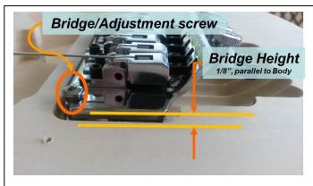
Fig 5.4 Action Adjustment
