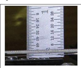
Fig 5.4 Pickup Height Measurement
