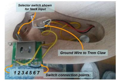
Figure 4.7.2-2 Body Wiring Tunnels
