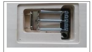
Figure 4.5-3 Tremolo Claw Installation
