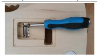
Figure 2.5 Tremolo claw Alignment
