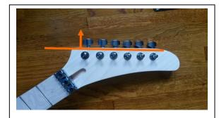
Figure 2.8 Tuner/Nut Alignment
