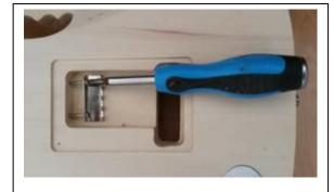
Figure 4.5-1 Tremolo Claw Installation
