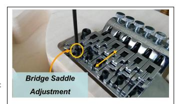
Fig 5.6 Intonation Adjustment
