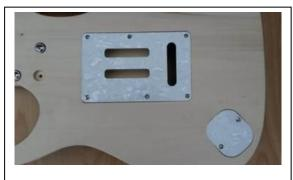
Figure 2.5.1 Back Body Cover Alignment
