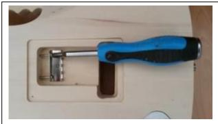
Figure 4.4.3-1 Tremolo Claw Installation
