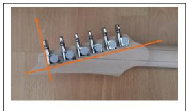
Figure 2.7 Tuner Alignment
