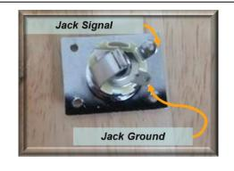
Figure 4.5.2-3 Output Jack Wiring Tunnels
