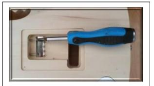
Figure 4.4-1 Tremolo Claw Installation
