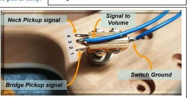
Figure 4.5.1 Selector Switch Wiring
