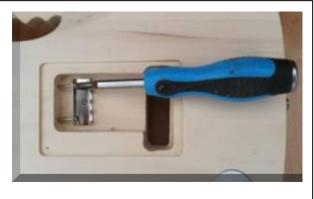
Figure 2.4 Tremolo claw Alignment
