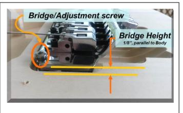
Fig 5.4 Action Adjustment
