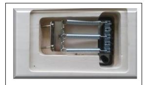
Figure 4.4-3 Tremolo Claw Installation
