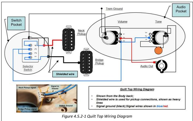
1. Starting in the Audio pocket and referencing Figure 4.5.2-2 for tunnel locations, run the two wires to the Bridge pocket;
